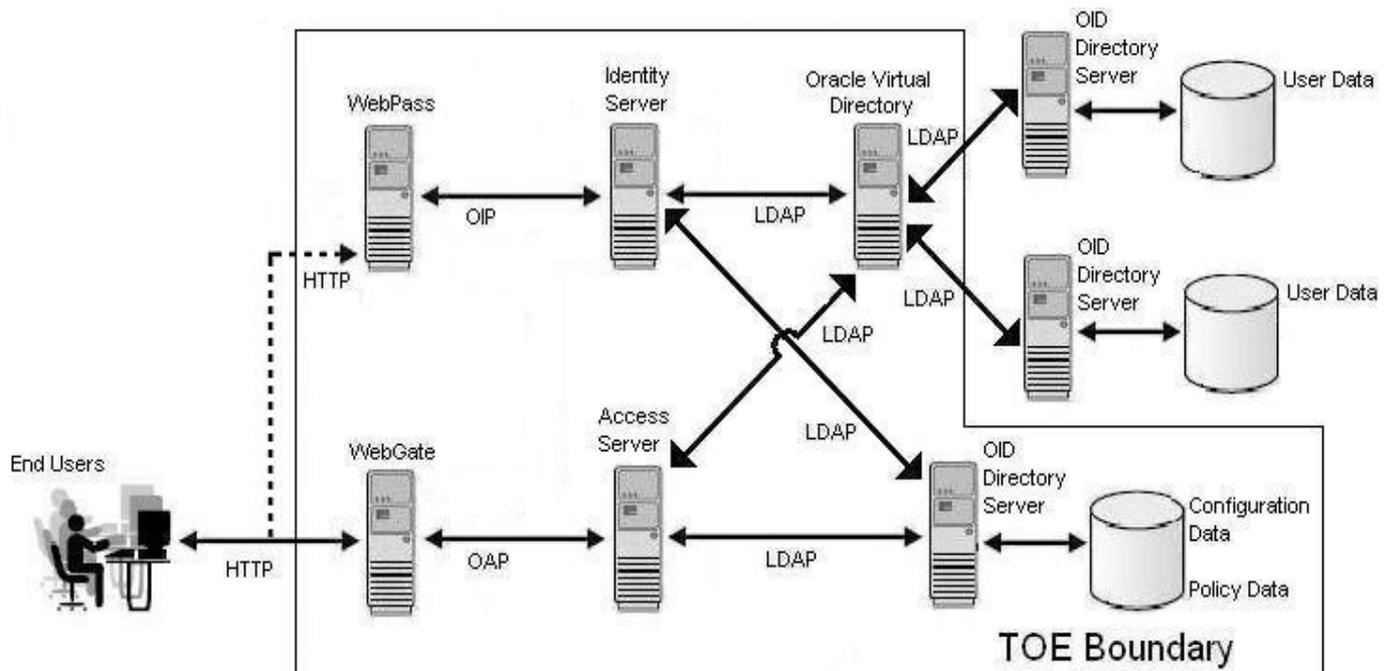
*Figure 2: TOE configuration*
